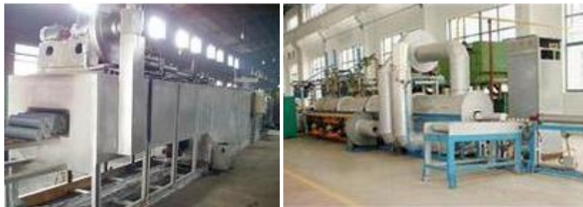
Application on aluminum rod heating furnace
